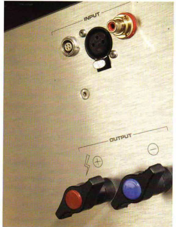
ABOVE: The Krell evolution 600 can accept a normal RCA unbalanced or XLR balanced input, or Krell's proprietary current source connection, via a four-pin connector
